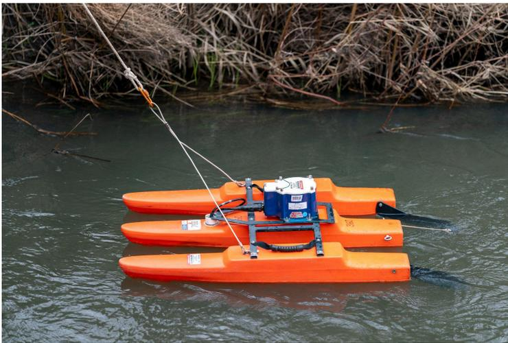
It is a device that uses sound waves to measure the speed and direction of currents through the water column. The National Oceanic Atmospheric Administration, for example, uses ADCPs to understand how water moves, which in turn provides important information about biological, chemical and physical properties of the ocean.
