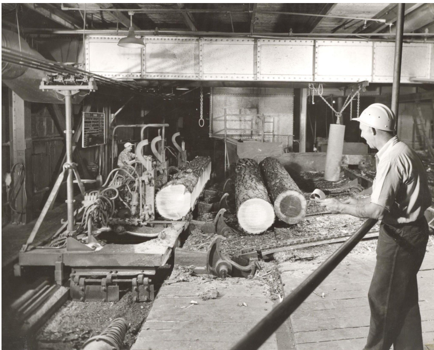
Pictured: Al C. Welcome at work inside Edward Hines Lumber mill. In the background, a man operates a head rig saw.
