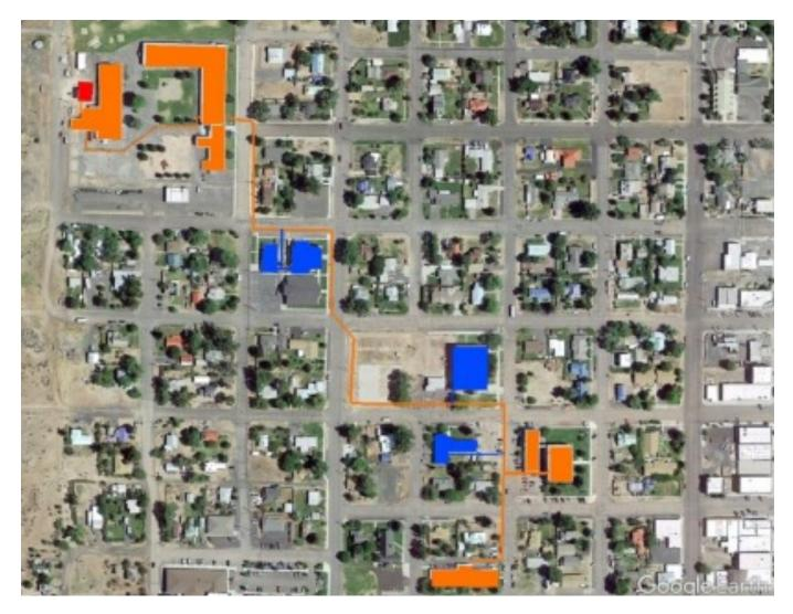
Biomass boiler (red); piping and connected buildings (orange); potential future connections with installed piping tees (blue). Graphic credit: Wisewood Energy
