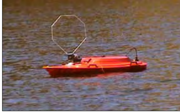
Figure R-22. Prototype of the robotic carp.
